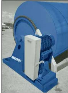
A Waconia Rotary Blender is marked by a cleaner, more professional, finished design. Heavy duty blender drive motors are totally enclosed, fan cooled and located in a higher relatively dust-free environment.
