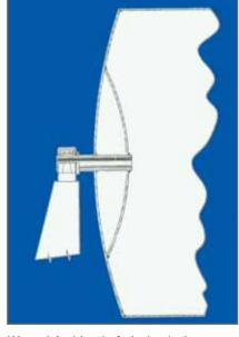
Waconia's driveshaft design is the strongest in the industry. Our huge 3-7/16" drive shaft intrudes a full six inches inside the blending drum where it is welded to a 30" diameter domed cap. This unique design distributes the weight and load of the blender across the entire width of the dome. The shaft is also welded to the outside of the drum and rides on a large pillow block ball bearing for more longevity.
