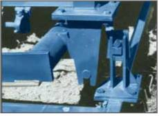
The Waconia weigh hopper is equipped with a modern knife and pivot pipe lever scale system for more durability and greater calibration accuracy. An electronic digital indicator that gives you much greater flexibility for weigh hopper placement, is optional.
