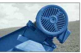
Waconia's weigh hopper conveyor features an exclusive hinged motor mount with a simple screw-type takeup that makes quick work of conveyor belt adjustment.
