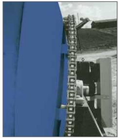
Drum drive sprocket features bolted construction for quick and easy replacement in the field.
